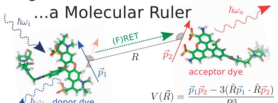
FRET distance measurements rest upon the RET theory developed by Theodor Förster. Assumptions in the theory yield a simple formula for the dye coupling potential V of the RET from donor to an acceptor dye. The formula allows the direct calculation of dyeto-dye distances R from efficiencies E. and thus the retrieval of spatial information [3]. FRET efficiency is measured e.g. by
