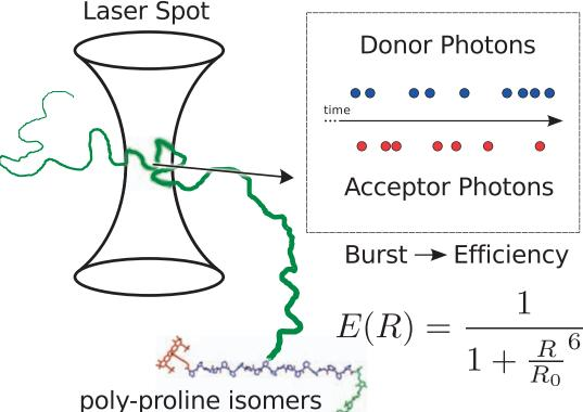
monitoring the relative weights the fluorescent decay channels from donor and acceptor. Although widely used in experiments, the approximations Förster's formula lead to a significant loss of  $\underline{R}$  6 accuracy in the distance measurement [1]
