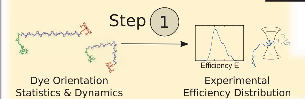
To overcome the  $\kappa^2$ -problem, we have combined experiments with MD simulations. Dye orientation statistics and dynamics from MD serves to calculate the orientation factor  $\kappa^2$  in the Förster formula for  $R_0$ . Moreover, distributions of  $\kappa^2$  from simulations are employed replacing a mean orientation factor in  $R_0$ .
