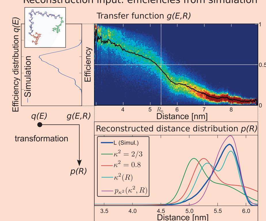
For the distance reconstruction, we developed a transfer function formalism in which the conversion of distances to efficiencies is given
