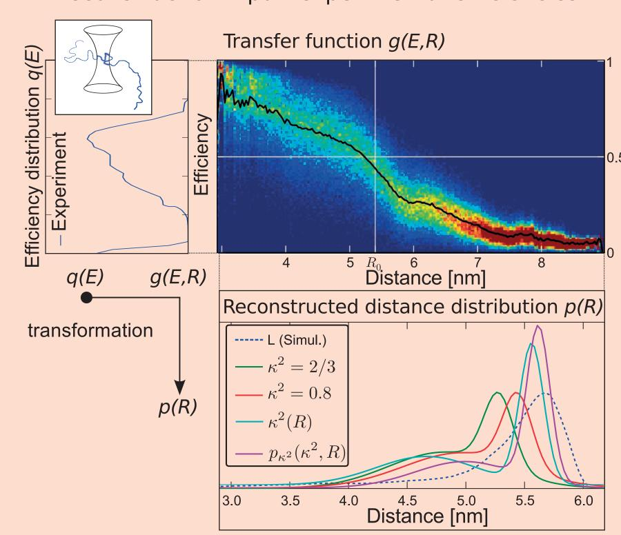
distances, respectively. The transfer function g(E,R) is refined for each approximation level. Inversion of the formalism allows calculation of distance distributions p(R) from experimental efficiency distributions q(E).
