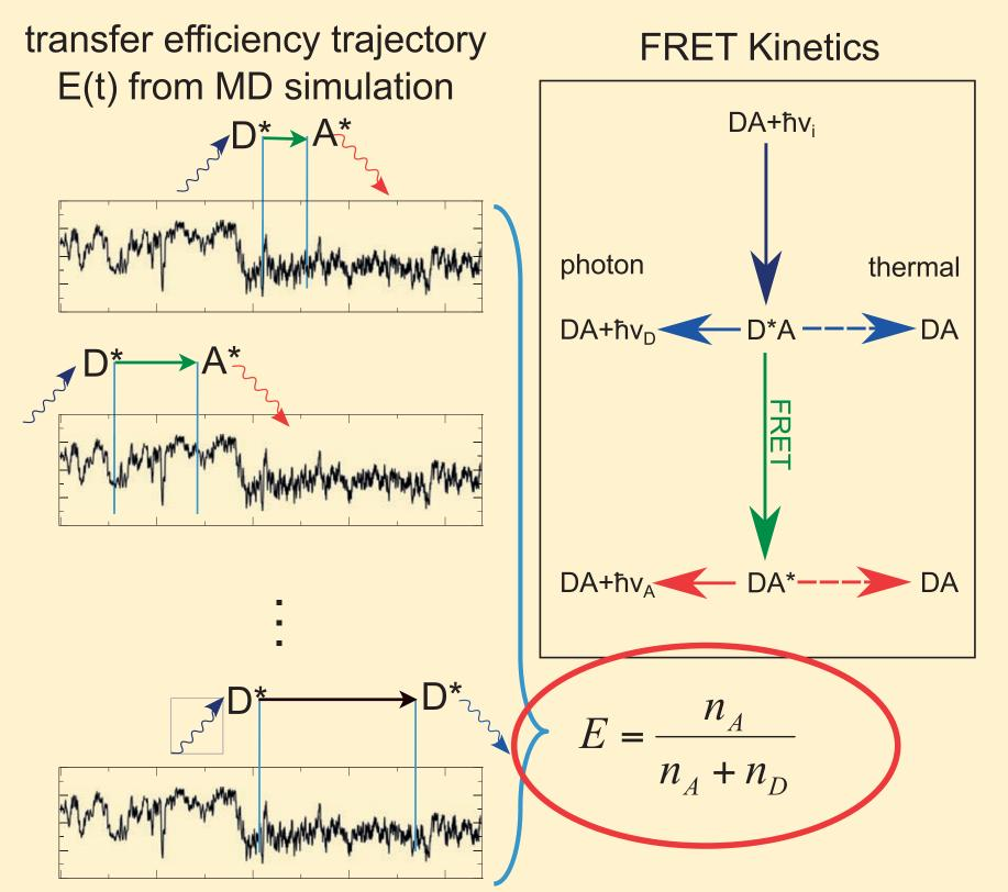
To calculate efficiency distributions from MD simulations, we employed a Monte Carlo (MC) approach to probe the kinetic pathways of FRET experiments. All probabilities in the kinetic scheme are considered as constant except the FRET probability  $p_T(t)$  which is calculated from the coupling between the dyes in the MD simulation and changes with every time-step.
